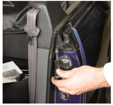
**STEP 2**Remove the door seal and pull the side panel forward,
